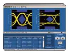
TDSRT-Eye™ software. Compliance and analysis for testing high-speed serial standards. Eye diagrams at data rates to beyond 6.25 Gb/s. Software clock recovery to ≥10 Gb/s.
