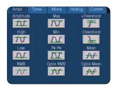
Measurement System. Enables over 50 parametric measurements in the amplitude, time and statistical domain.
