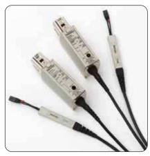
► P7313 12.5 GHz and P7380 8 GHz Differential Probes.
